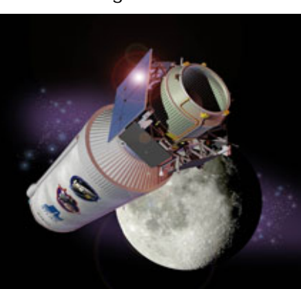
The LCROSS S-S/C attached to the Centaur rocket. The S-S/C will follow the Centaur to the surface after their separation. Photo courtesy NASA
